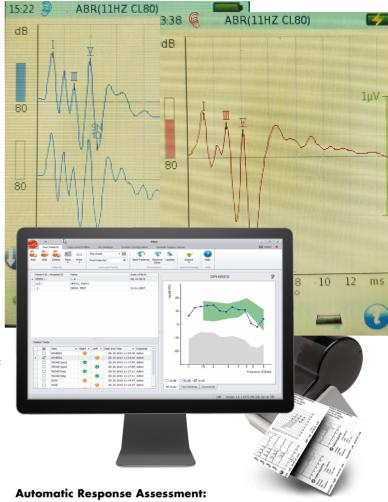
The software labels recordings automatically as Probable or no-response as they are acquired, based on advanced detection algorithms..
